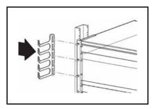
3 Tighten the screws to secure the guide to the chassis.
